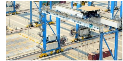
Fully-electric ASC/ARMG (cable reel)
