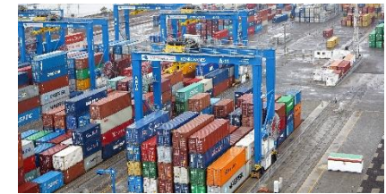
Fully-electric ARTG (cable reel)
